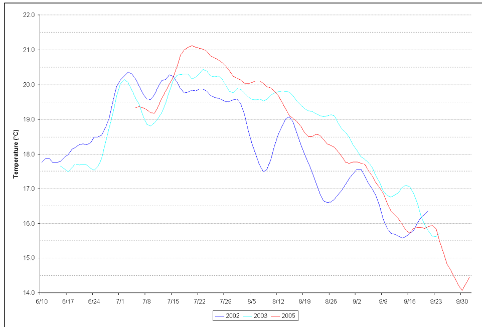
Figure 2-4. Summer 7- Day Rolling Averages Of The Daily Average Temperature (2002, 2003, 2005, 2007) Near The Downstream Property Boundary (Wheel Gulch). The Highest 7-Day Peak Of The Rolling Average Is The Annual MWAT.
