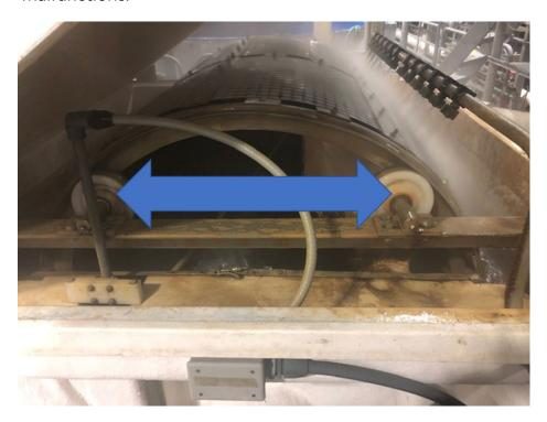
**Figure 9**. Drum filter support wheels indicated by the double-sided arrow.
